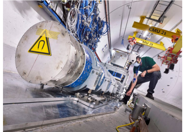
The FASER particle detector, located deep underground at CERN's Large Hadron Collider and built-in large part out of spare parts from other experiments'
